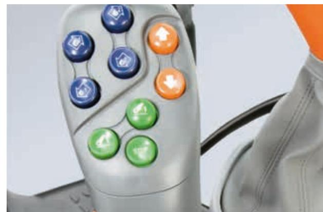
The Powershift stages can also be shifted at a touch with the PowerCom5 operating lever.
