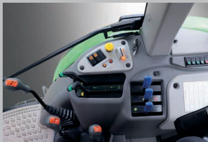
Electro-hydraulic engagement for PTO differential lock and 4WD.
